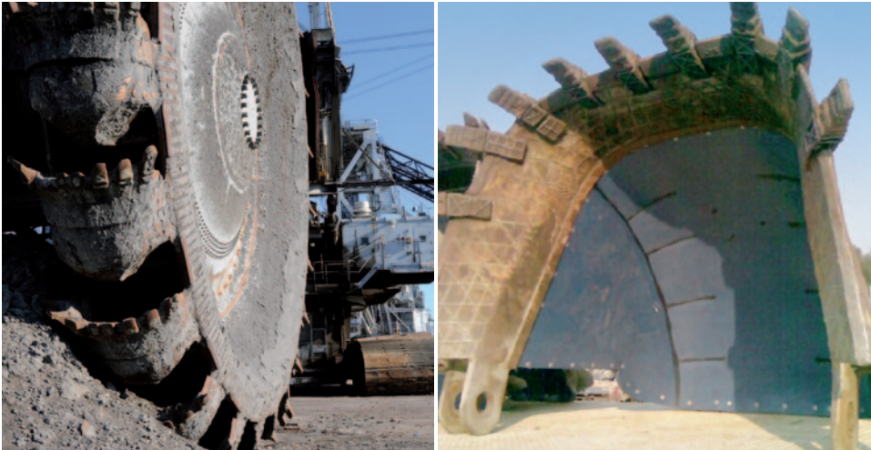
Open-pit coal mining buckets in Australia lined with dehoplast® superlining.
