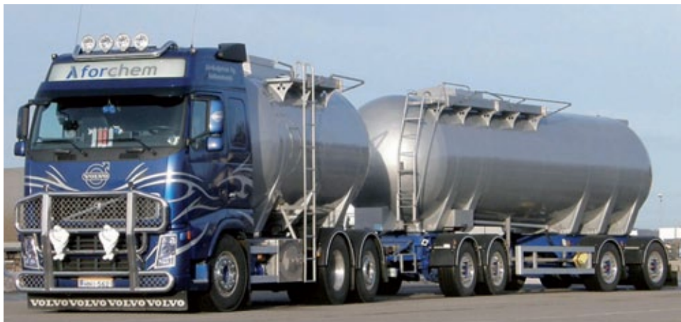
18 m³ and 31 m³ road tankers featuring 2.3 mm SIMONA® E-CTFE-AK in a dual laminate design
