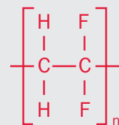
Fig. 2: Partially fluorinated plastic, e.g. PVDF (polyvinylidene fluoride)
