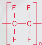
Fig. 3: Fully fluorinated plastic, e.g. PTFE (polytetrafluoroethylene)
