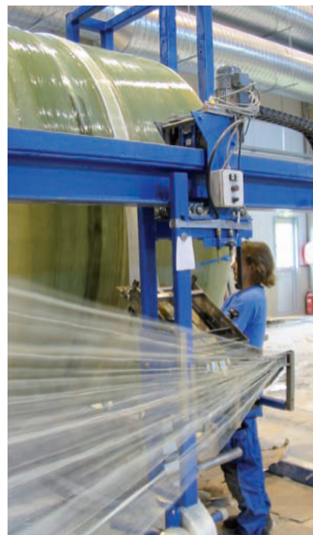
Creating the GRP structure by means of filament winding (onto the liner material SIMONA® E-CTFE-AK)
