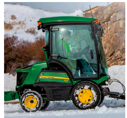
John Deere tractor engine cover made with PMC® StrataGem™
