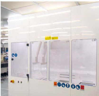
Body of a wet-processing unit made of SIMONA® PP-H white sheets
