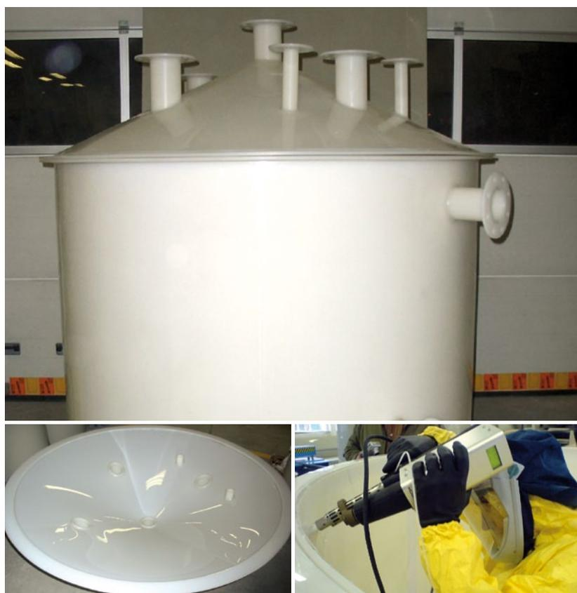
Above: Finished tank. Below: Roof of the tank made of PVDF sheets 8 mm thick. Welding the PVDF semi-finished products.
